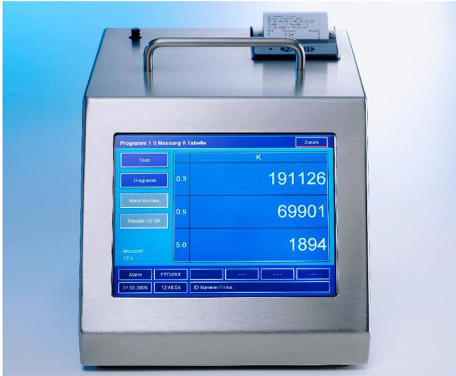
The **PZG** line with a flow rate of 100 LPM offers a sensitivity of 0.3  $\mu\text{m}$  (micron) (Alternative: 28.3 LPM = 1.0 CFM with a sensitivity of 0.2  $\mu\text{m}$ ) and is available in three types:
